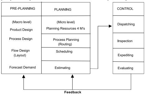
Fig. 5.2 Functions of production planning and control
