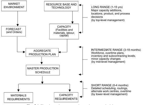
Fig. 5.4 Flowchart of aggregate plan and master schedule
