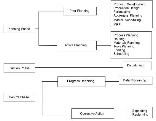
Fig. 5.1 Phases of production planning and control
