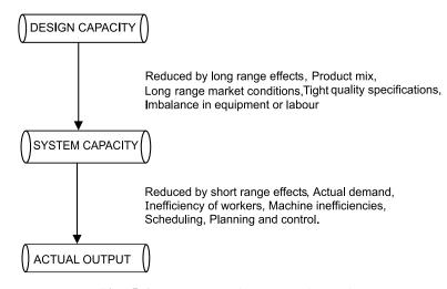
Fig. 5.6 Capacity and output relationship
